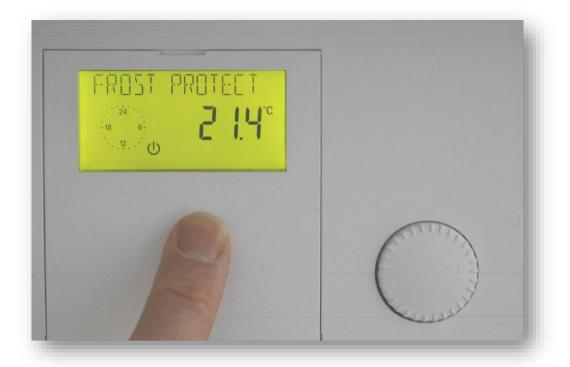
Note the display indication and select your required parameters using the rotary selector at the corresponding point (Standby/Automatic/Day or setback mode/DHW heating/Emergency mode).
