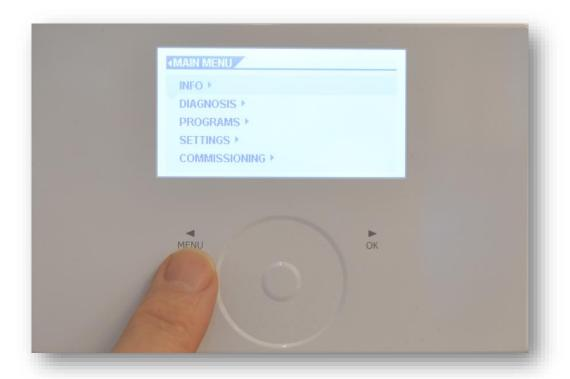
Move your finger clockwise around the scroll wheel until the bar is on COMMISSIONING. Then press OK
